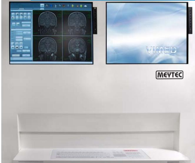
The left upper picture shows the cockpit with two displays to perform diagnostics (left) and electronic recording of patient data / video communication. The right picture shows controls of the CT-lock, the CT-control monitor and the CT-emergency stop switch.
